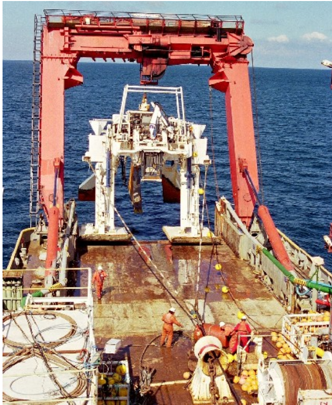
Figure 3.6 A plough is lowered into the sea from the auxiliary vessel (source: Metoc)
