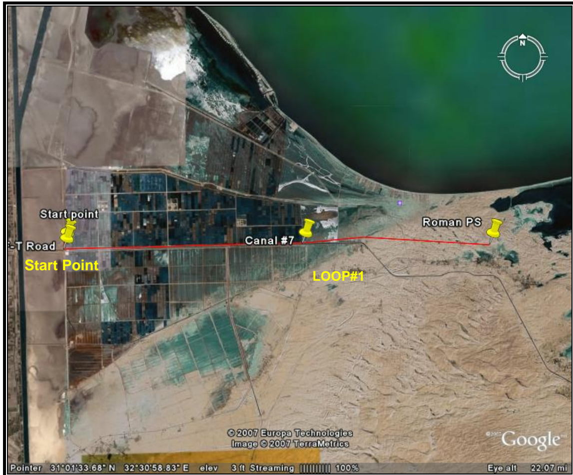
Figure 6.2. “KM point 00+00 to KM point 23+00 shows the proposed route penetrating extensive reclaimed agricultural area (in the vicinity of El -Sheikh Gaber Canal) and crossing four branch irrigation canals No. 1,3,5,7
