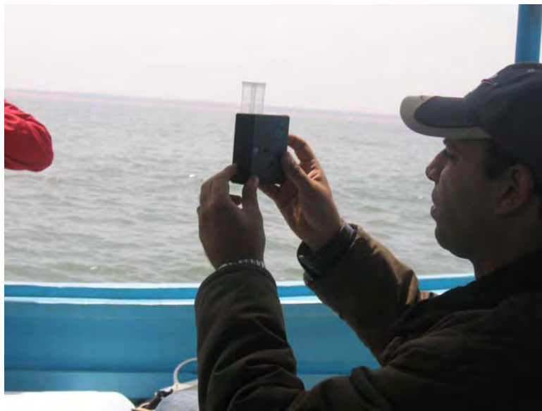
Plate 6: Onsite Chlorine Analysis
