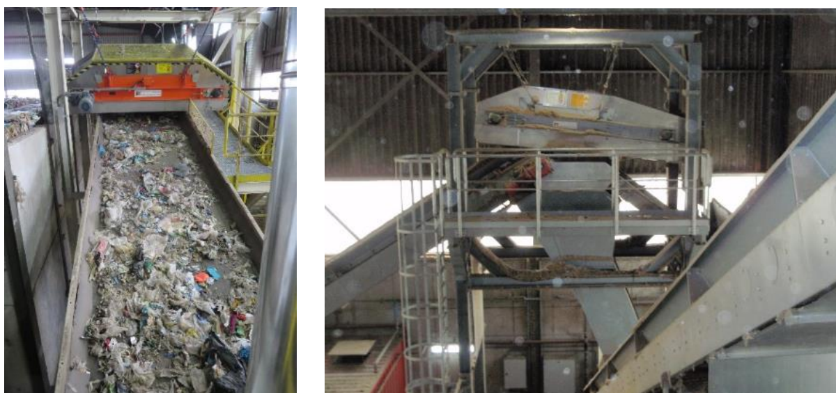
Figure 14: Left: A magnetic separator across the conveying direction in an RDF plant (less favourable position). Right: Favourable positioning of a magnetic separator parallel to the conveying direction and at the discharge point of the left conveyor belt
