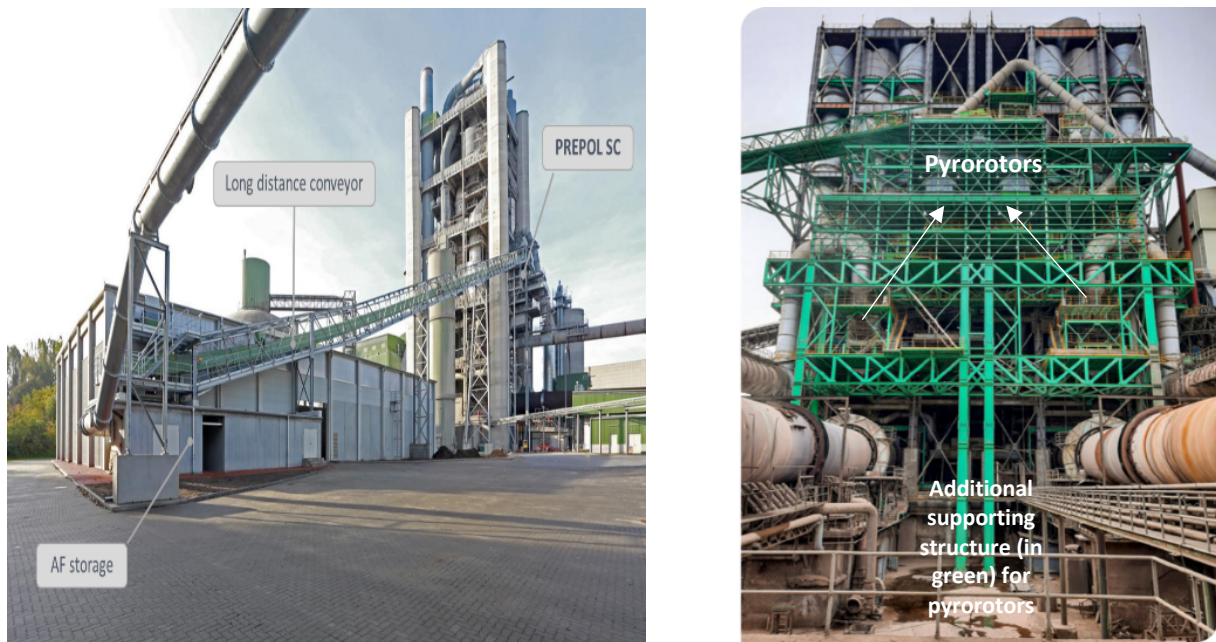
Figure 34: Left: Installation of Prepol SC by Thyssenkrupp in a cement plant in Germany. Right: Installation of Pyrorotor by KHD in a cement plant in South Korea
