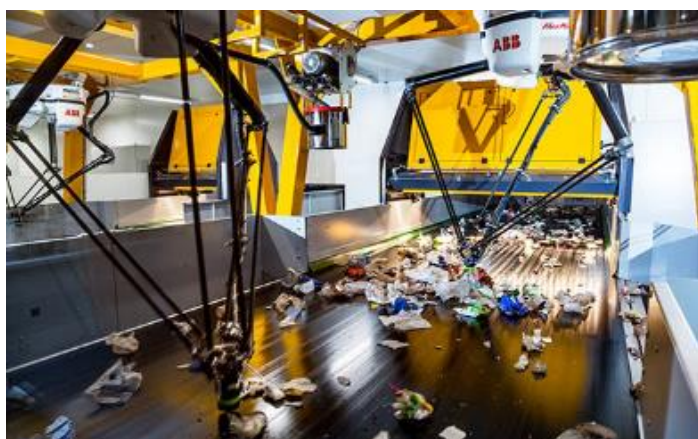
Figure 30: Sorting robots in action
