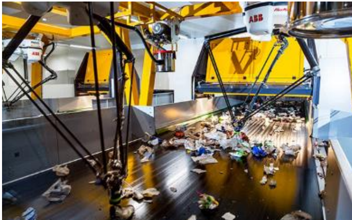
Figure 30: Sorting robots in action
