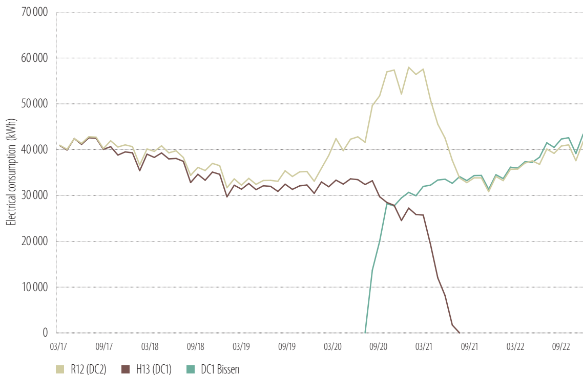
Figure 10: Electricity consumption of EIB Group data centres (kWh)
