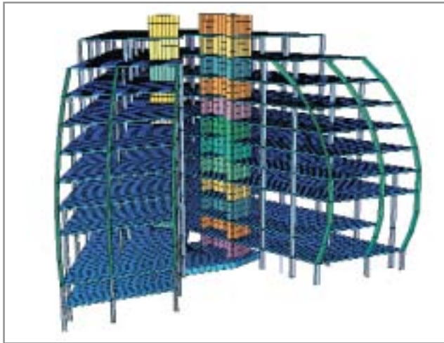
Concrete Structure - Finite Element Model
