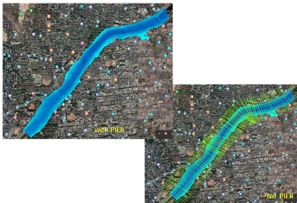
Figure 2: Inundation extent coverage with and without metro piers at the 1.45km stretch (source: CPWRS Report, 2021)
