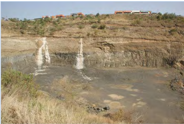
Basalt Quarry No.2 ready for closure. Rehabilitation will involve smoothing slopes, top soil application and revegetation
