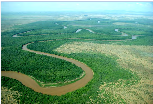
Typical profile of the Omo valley in the plain (chainage km 350-660). Intense meandering, recession agriculture, oxbow lakes inside meanders
