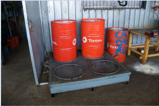
Mobile storage device for hazardous materials
